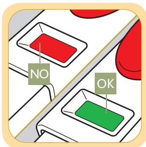
The indicator turns green when it has been anchored correctly
